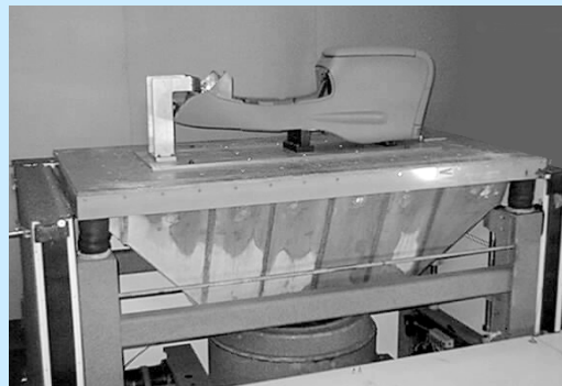
Figure 32-17D Massive Fixture drives Console Specimen
