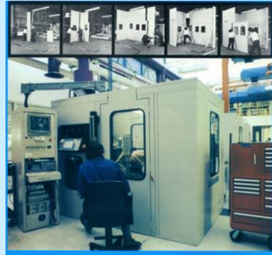
Figure 32-22 Erecting a "Quiet Room" Inside a Factory
