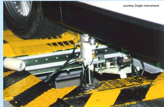
Figure 32-12 Energizer docked to car body
