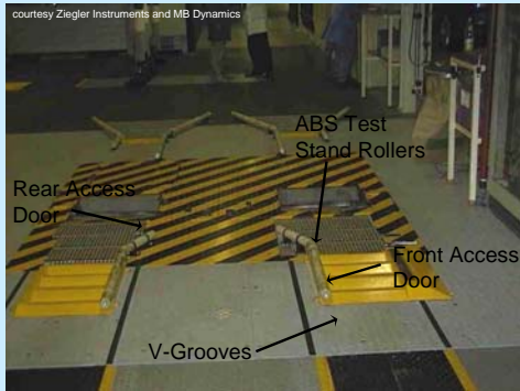
Figure 32-11A Floor Level of Prufstand
