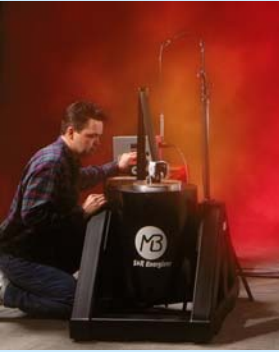
Figure 32-22A Seat Belt Retractor BSR Investigation inside a "Quiet Room"
