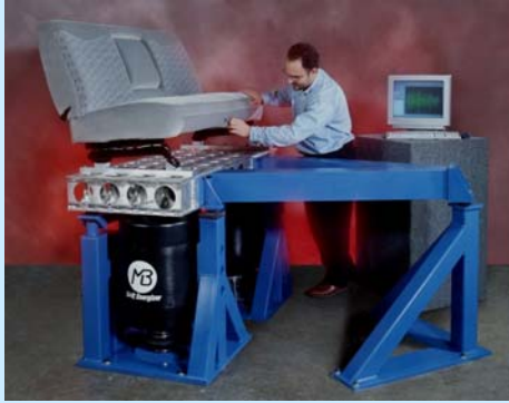
Figure 32-18 Seat Assembly on two ED Shakers
