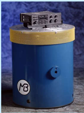
Figure 32-17A Quiet ED Shaker for BSR Investigations
