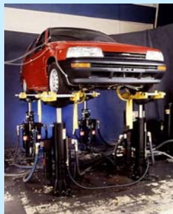
Figure 32-9C - “Four Poster” shaking for BSR investigation
