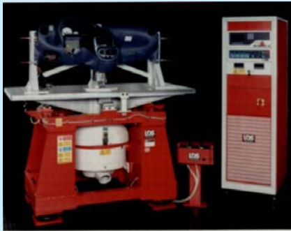
Figure 32-14 A Instrument Panel on ED Shaker
