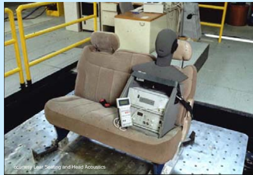
Figure 32-3 Automotive “Sound Quality” Apparatus
